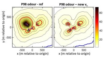
Figure 2. The 98-percentile of all 2015 hourly values for odour (Odour Units m<sup>-3</sup>) for the poultry reference case ( $v_s = 0.4 \text{ ms}^{-1}$ ) and case with new exit velocity ( $v_s = 5.5 \text{ ms}^{-1}$ ). The red and blue contour lines represent 14 (standard rural area) and 3 OU m<sup>-3</sup> (standard built-up area) respectively. The blue circles represent the included sources.
